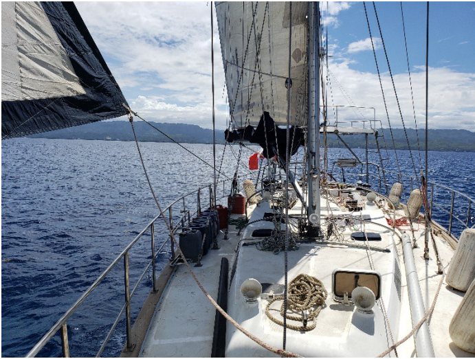
MACH 1 has solid railings, large deck, excellent standing rigging, 6 dorade vents and hatches (polycarbonate replaced).
